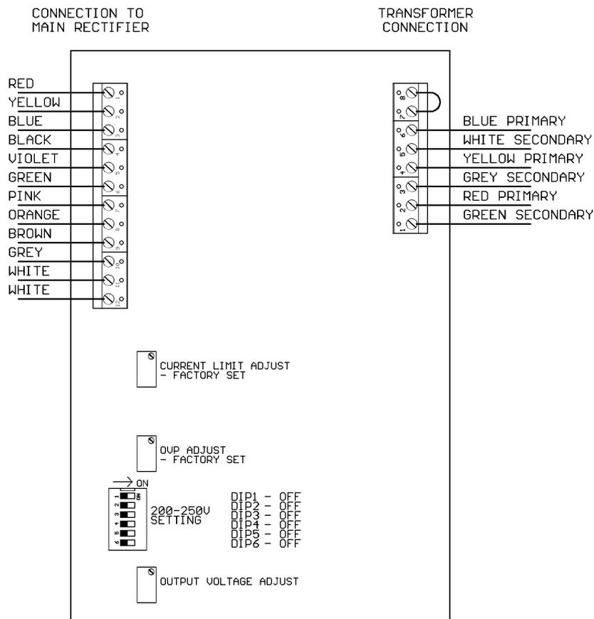
REMOVE BRIDGE CONNECTION K1-K2 ON MAIN RECTIFIER BOARD IF PRESENT
