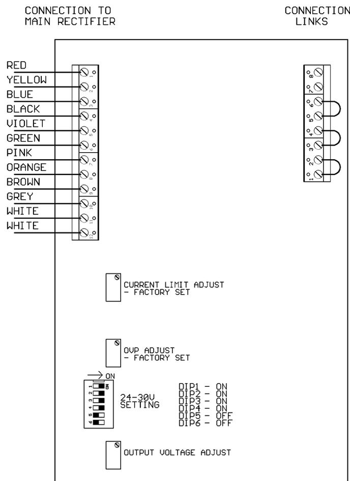
REMOVE BRIDGE CONNECTION K1-K2 ON MAIN RECTIFIER BOARD IF PRESENT
