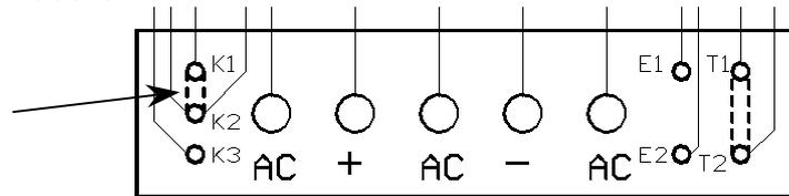
If it is necessary to have an off-switch, a 3-poled switch must be used rated for 4-10 Amp. It should be connected so it breaks the transformers primary connections in a 110/220 Volt system and so it replaces the three links in a 24 Volt system.
